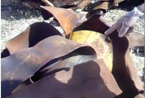
**Appendix 17**The remnants of a toxic chemical cylinder. Note that the cylinder has ruptured at the nose end.
