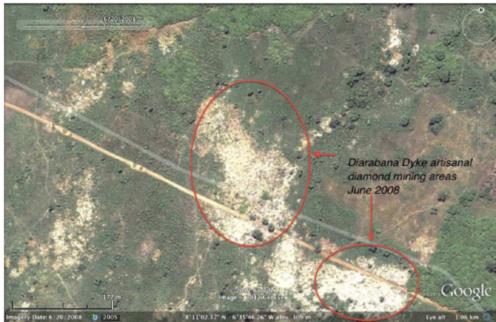
Diarabana dyke – the area after three years of artisanal exploitation with the dyke line now becoming distinctly evident.
